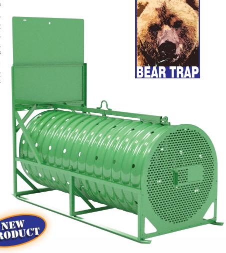
A sliding dart door is conveniently located on the back panel to help safely subdue the animal inside. Multiple vents have been drilled out of the culvert tube and are also laser cut from the back panel for better air flow. Small drain holes have also bee drilled out of the bottom of the culvert tube. For animal safety, all bolt heads face inside and all nuts and bolt ends protrude outside the trap.
