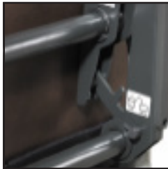
Lock - automatically engages when the tabletop is moved into the full upright position to prevent accidental shifting in storage.
